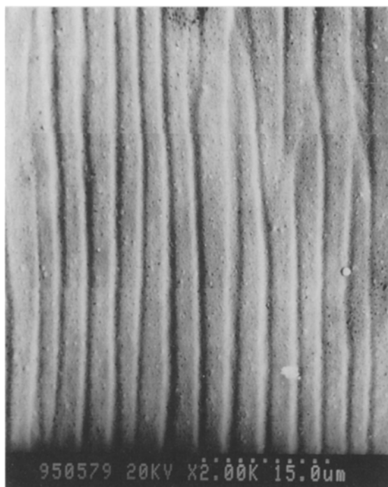
Figure 2. SEM micrograph of the sheared HPC film. The pleat period is about 4\ \mu\text{m} .
